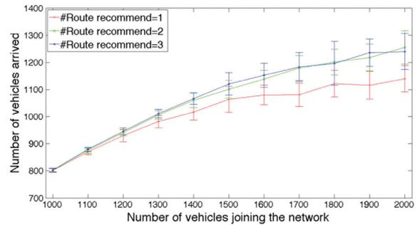
Fig. 2. Number of vehicles arrived at destination in 1 hour
